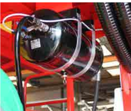
Tank with overpressure safety
