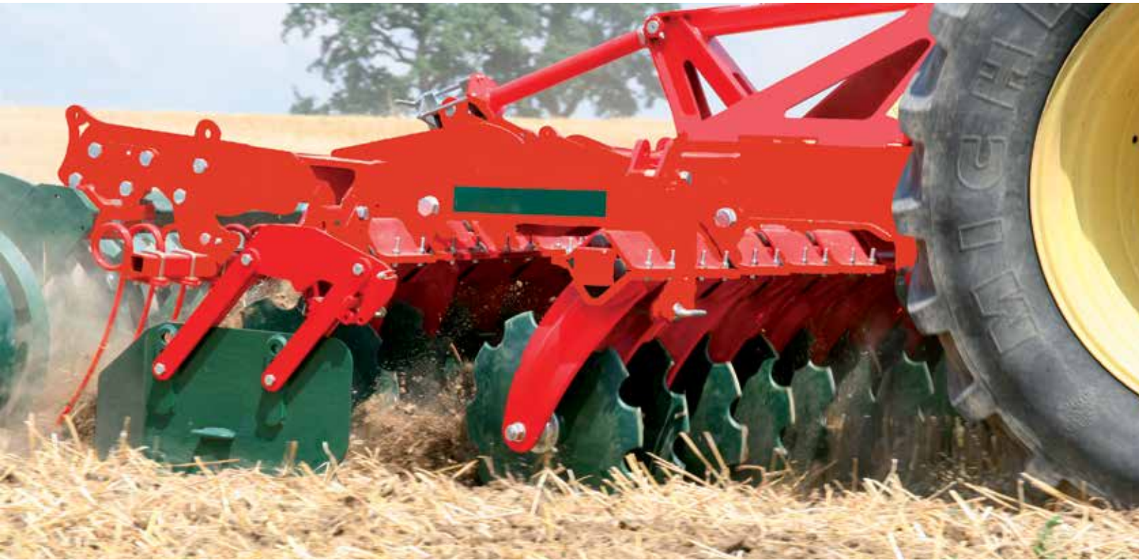
Aggressive disc form and position guarantee very good introduction and best incorporation
